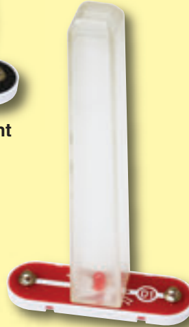
Light Tower LED attachment mounted to D1
